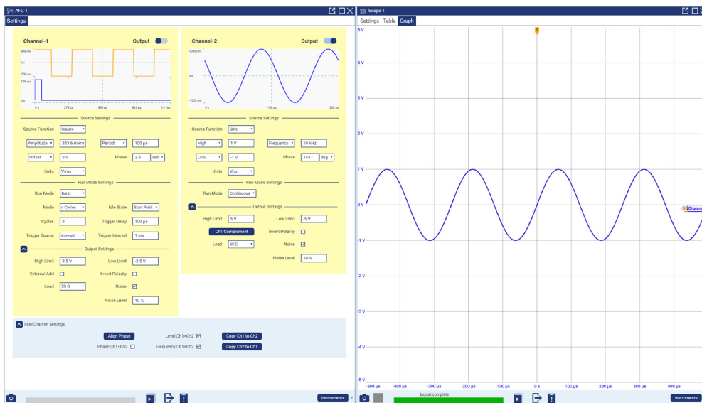
Use the Scope App to capture data sourced using the AFG App
